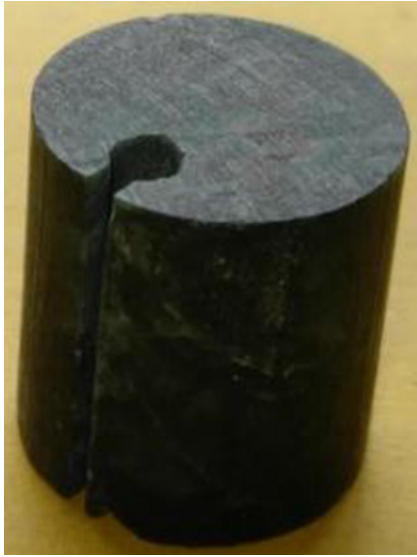
Fig. 7. Slug after machining for solution No. 2 from set of Pareto optimal solutions provided in Table 9.
