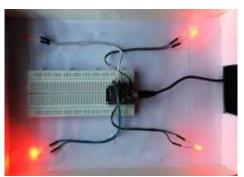
Fig. 3: Automation using ESP8266 NodeMCU
