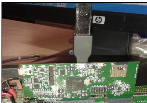
Fig. 5 TI's F28377D ControlCard
