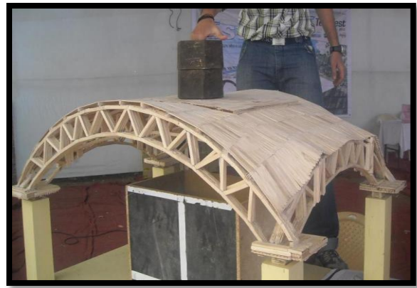
Fig.3. Testing of Shell Structure Model
