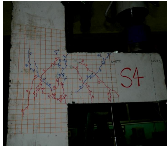
Fig. 10 Crack Pattern of Specimen S4
