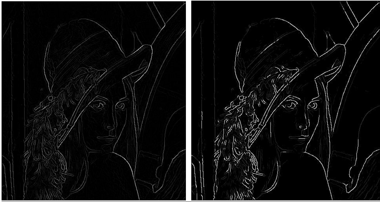
Fig 14 : Threshold result: weak pixels in grey and strong one in white.
