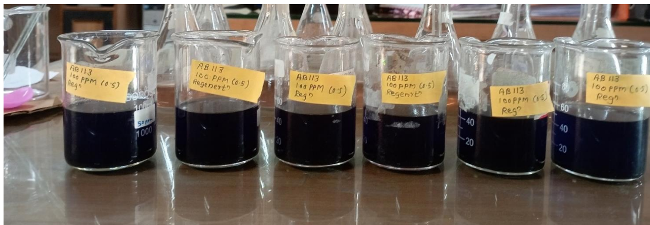
Fig. 5.6a Desorption study using ethanol as desorbing agent
