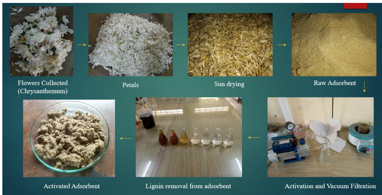
Fig. 4.2 – Overall process of biosorbent synthesis
