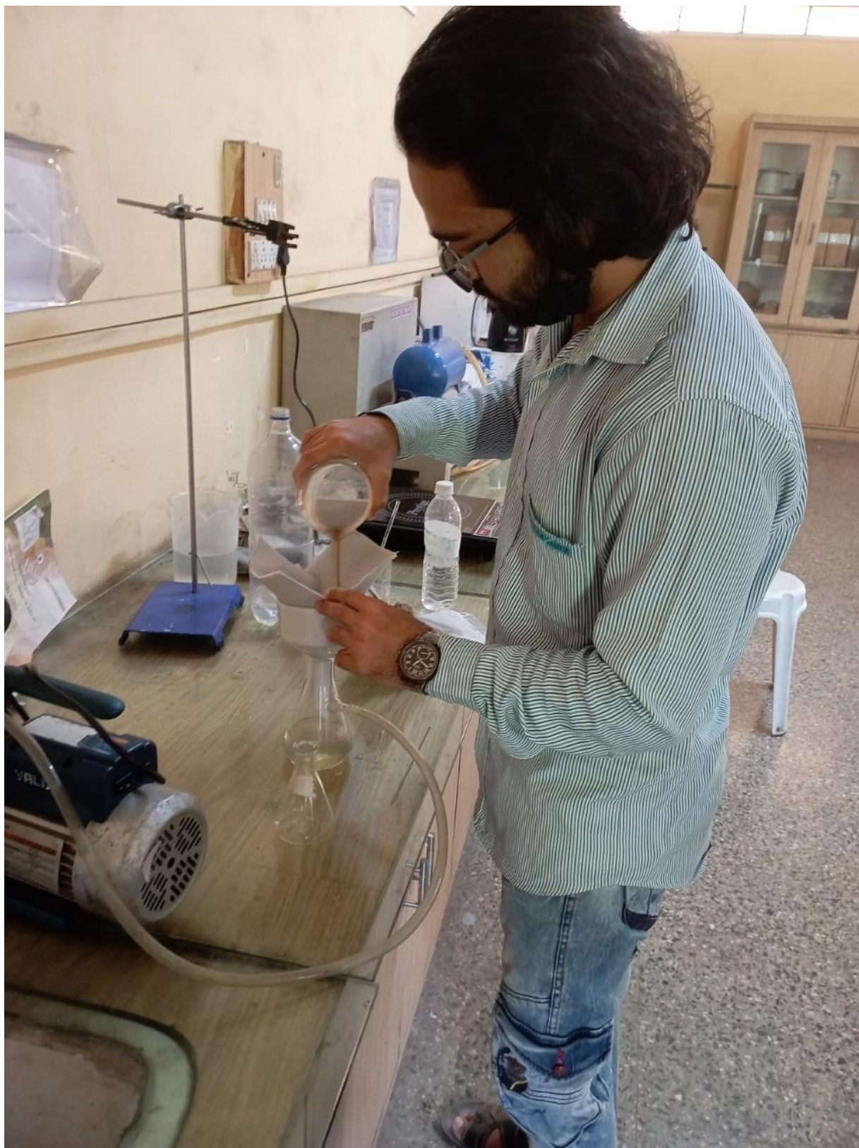
Fig. 4.4 Experimental image of vacuum filtration for biosorbent activation
