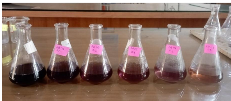
Fig. 5.3a Biosorbent dosage experimentation image showing removal of AB113
