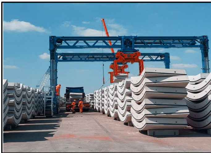
Fig. 3.21: Precast tunnel segment stacking yard
