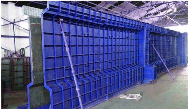
Fig. 3.12: Site-specific formwork system
