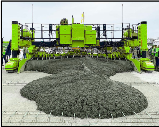
Fig. 3.16: Slip-form paver for concrete pavements
