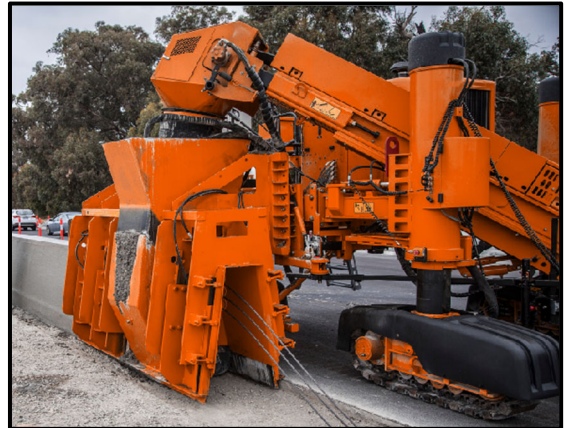
Fig. 3.17: Slip-form for concrete medians
