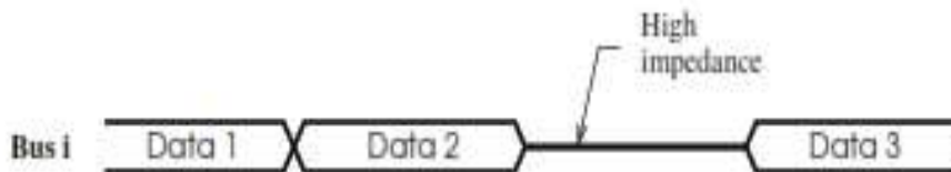
Fig. 7.7: Data representation on a bus
