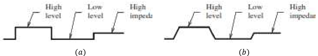
Fig. 7.6: Representation of a signal: a) ideal case; b) considering the rise and fall times
