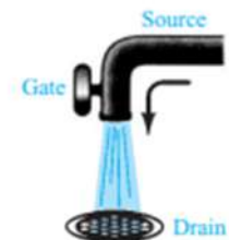
Fig 5.5: Water Analogy for the JFET
