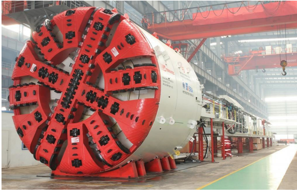
Figure 5: TERRATEC EPB TBM used for tunneling in the Delhi Metro (Source: https://tunnelingonline.com/ )
