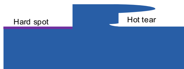
Fig. 2.23 Schematic showing localised hard spot formation and hot tears
