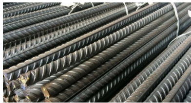
Fig. 1.16: Typical HYSD (High yield strength deformed) bars
