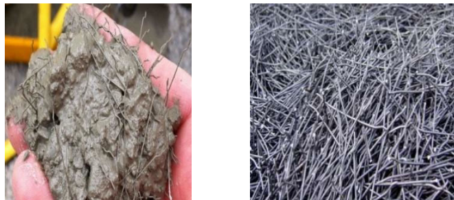
Fig. 1.7: Steel Fibre Reinforced Concrete and steel fibres (References: Civiconcepts.com; Behbahani et al. 2011)
