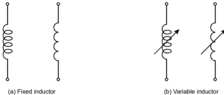
Fig.1.7: Symbols of fixed and variable inductors
