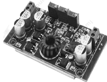
Fig. 5.16: Pictorial view of a buck-boost converter
