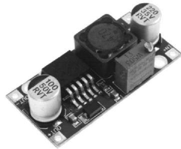
Fig. 5.9: Pictorial view of boost converter
