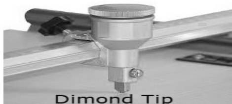
Fig. 4.40: Conventional Glass Cutting Method
