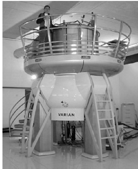
NMR Magnet at Birmingham, UK, with strong 21.2-tesla field, proton resonance is at 900 MHz
