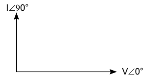
Fig. 5.17: Phasor Diagram a pure capacitive circuit
