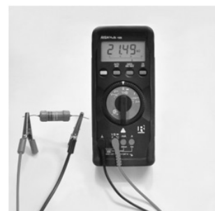
Fig. P13.2: Resistance Measurement using Digital multimeter
