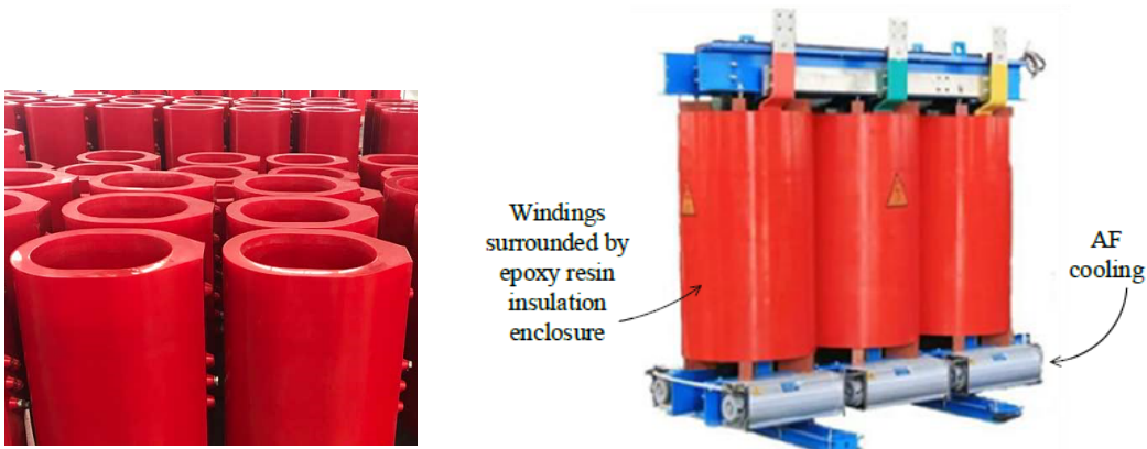
(a) Epoxy resin insulation enclosures (b) 3-Phase, 1250 kVA, 11kV/433 V, cast-resin, dry-type, indoor distribution transformer,
