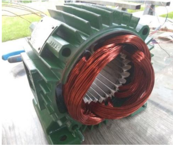
Figure 2.4 Rewinding 3-Phase Motor (Source: https://www.instructables.com/Rewinding-3-Phase-Motor/ )
