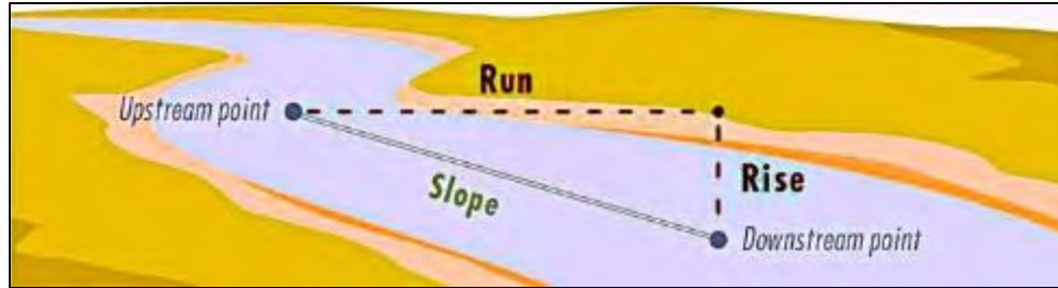
Figure 2.15 Measurement of slope of a stream
