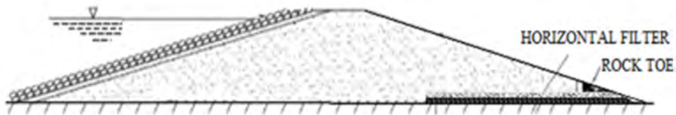
Figure 3.8 Horizontal filters to control Seepage in Dams
