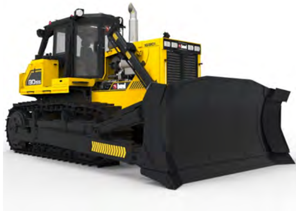
Figure 1.5: A hydraulic crawler dozer makes use of hydraulics to generate tremendous forces which help in earth moving operations. https://www.bemlindia.in/product/bd155/ .
