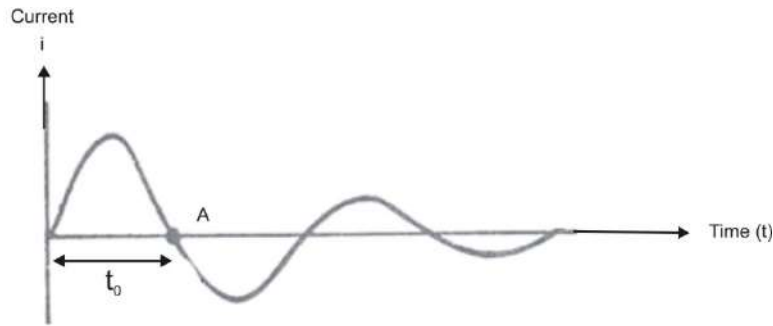
Fig.3.18 Current flows through SCR in Class A-series resonant commutation
