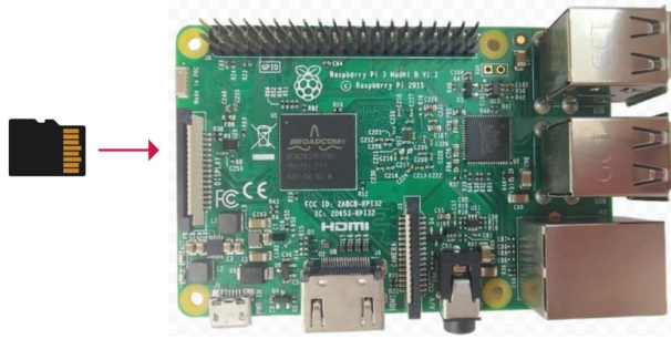
Figure 4.3: Location of SD Card in Raspberry Pi
