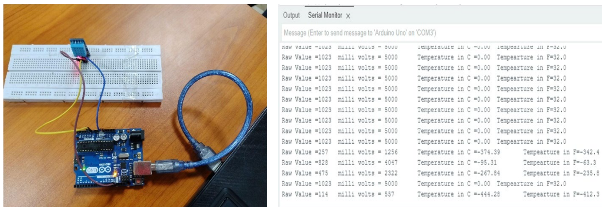
Figure 3.27: Temperature Sensor with Output on Serial Monitor
