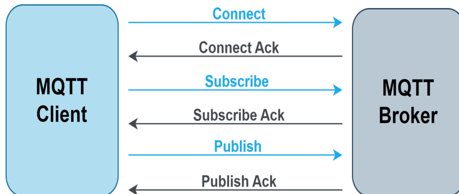
Figure 2.6: MQTT Message Flow
