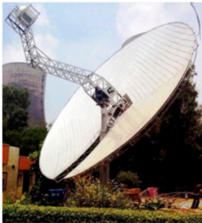
Fig.3.45 Circular Paraboloid dish (90 m 2 & 55 m 2 collector Area by Megawatt Solution) [Image Source: Megawatt Solution]
