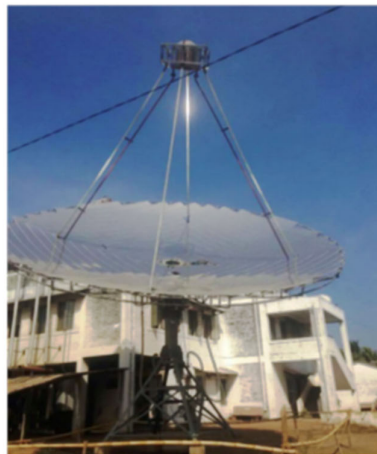
Fig.3.45 Circular Paraboloid dish (90 m 2 & 55 m 2 collector Area by Megawatt Solution) [Image Source: Megawatt Solution]
