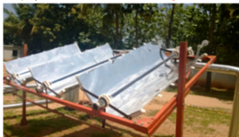
Fig.3.38 PTC ( 1.7\text{m}^2 ) by Oorja Energy
