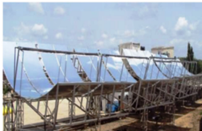
Fig.3.34 Large Aperture Parabolic Trough SharperSun ( 29.22\text{m}^2 ) by Leveragenet
