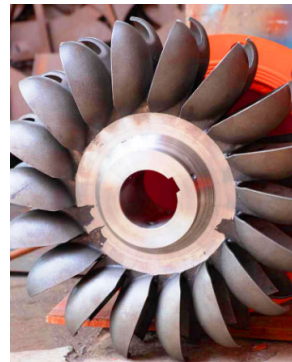
Fig.2.20 Pelton turbine
