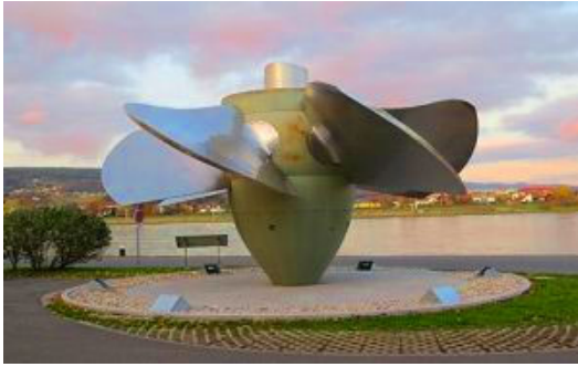
Fig.2.25 Kaplan turbine
