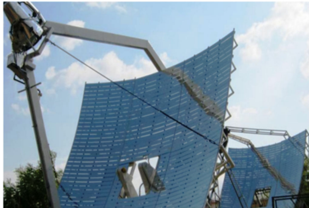
Fig.3.44 Square Paraboloid dish (25 m 2 collector Area by ATE Enterprises) [Image Source: ATE Enterprises website]
