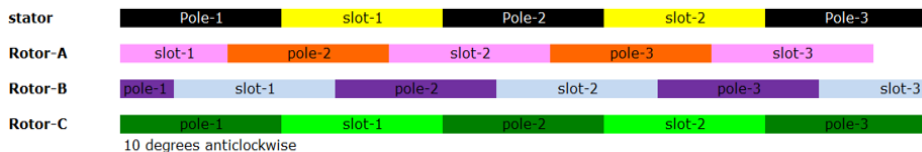
Fig.8.30: Operation of 3-stack stepper motor
