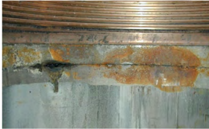
Fig. 5.6: Oil and gas pipeline under crevice corrosion
