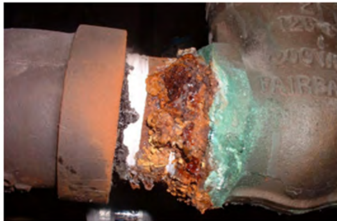
Fig. 5.5: An example of galvanic corrosion in oil and gas pipelines
