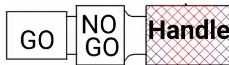
Figure 1.10 Progressive Plug Gauge
