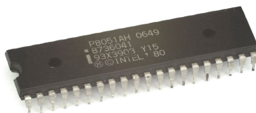
Fig. 2.7 Intel P8051 Microcontroller
